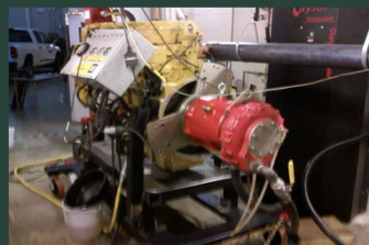
CAT 3176 diesel engine mounted on 3100 Taylor water break dynamometer
